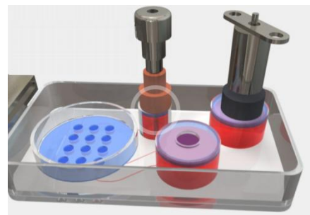
Figure 2. Valve for fluidic control and sampling compartment for pH measurements
